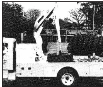
10. A service truck with a hydraulic hoist is essential to installing and removing today's heavy off-the-road tires.
