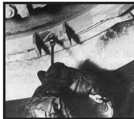
Running wire through the stem of an single piece wheel.
