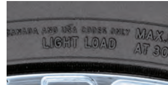
Figure 1—Light Load molded into sidewall
